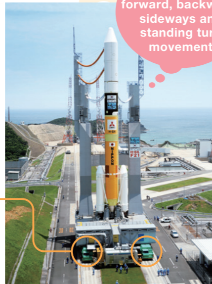
Dolly's power generation system also supplies electricity to the loaded satellite.
