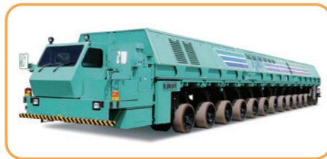
Dolly's power generation system also supplies electricity to the loaded satellite.
