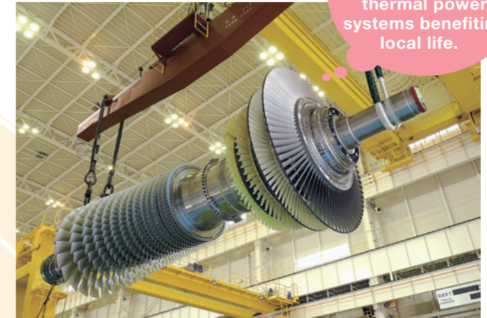
A key product — the gas turbine: The J-series gas turbine incorporates unique MHPS technology and ranks among the world's top class in power generation efficiency with a fuel-to-power conversion rate of more than 60%.
