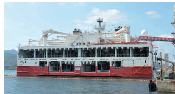
Stern of the RAMFORM TITAN. The streamer deck at the vessel's stern can house 24 streamer cables.
