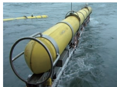
Air sources produce acoustic waves that bounce off the seabed and are picked up by sensors.
