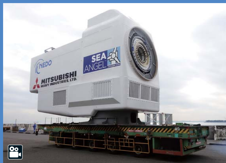
Demonstration unit "MWT100H" being tested at Yokohama Dockyard & Machinery Works (photo right). The unit's nacelle holds a hydraulic drive train (photo above).
