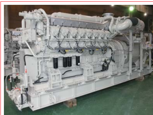
Heart of the MEGANINJA: a high efficiency gas engine (1,500kW)
