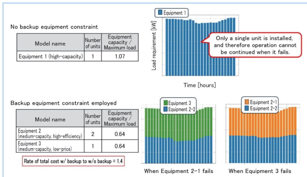
Figure 4 Results of equipment configuration optimization employing backup equipment constraint
