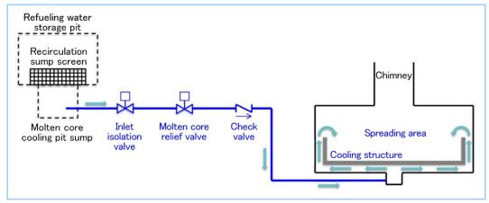
Figure 3 Gravity injection into spreading area
