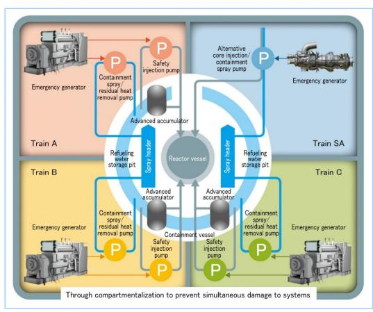
Figure 4 Concept of compartmentalization
