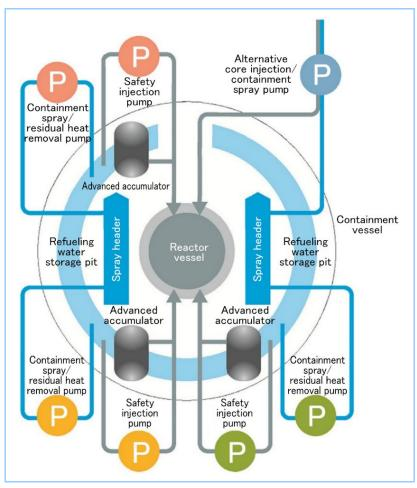
Figure 1 Configuration of triple-redundant safety systems
