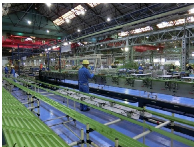
Figure 3 Assembly using large stationary jig
