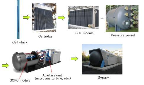
Figure 2 Composition of hybrid system
