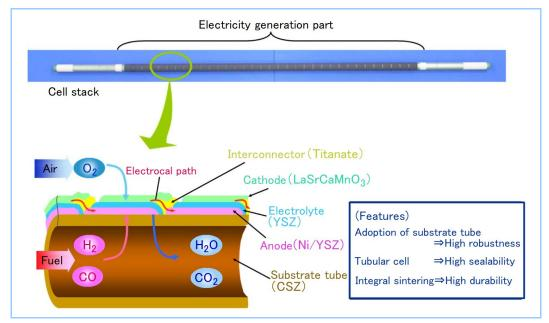
Figure 1 Structure of cell stack
