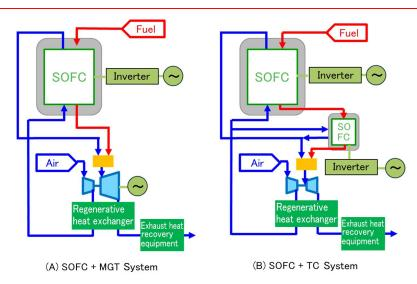
Figure 3 Comparison of MGT system and TC system
