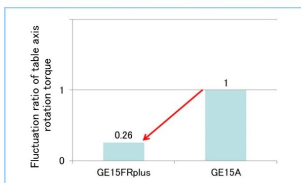
**Figure 4** Comparison of table axis rotation torques
