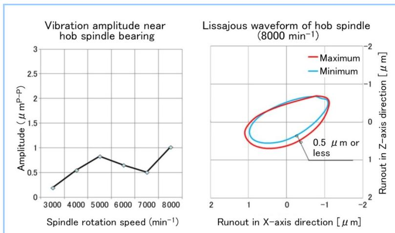
**Figure 3 Vibration amplitude near hob spindle and Lissajous waveform of hob spindle**
