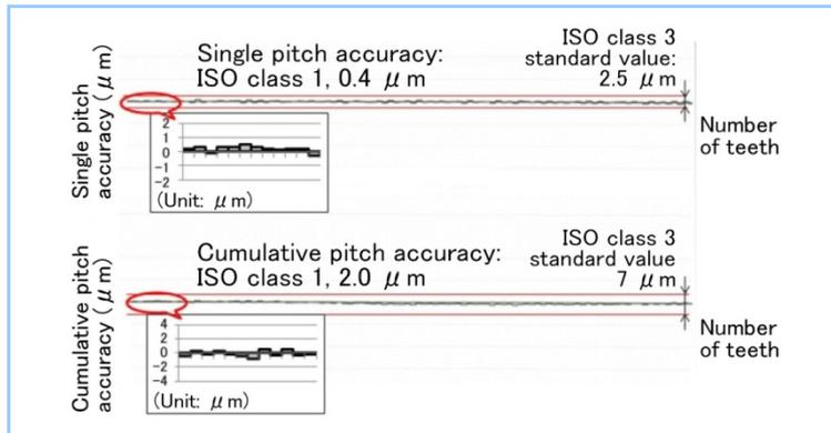
**Figure 6** Results of pitch accuracy machining with GE15FRplus
