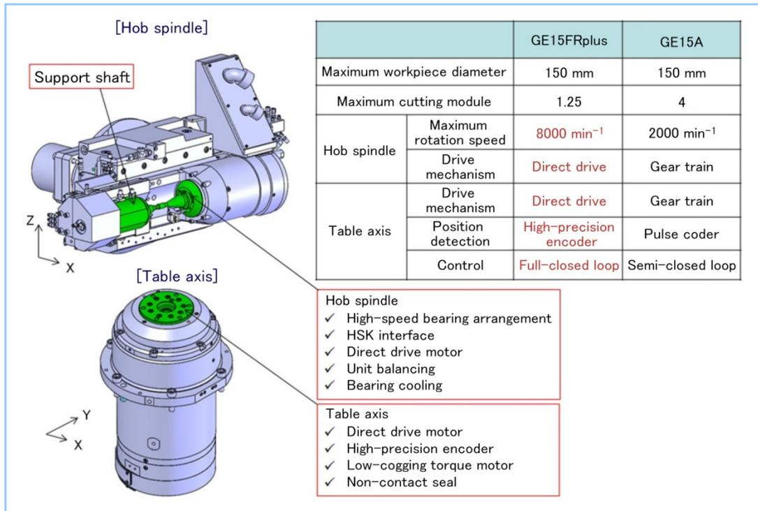
**Figure 2 External views and mechanical specifications of GE15FRplus hobbing machine, including features of hob spindle and table axis**
