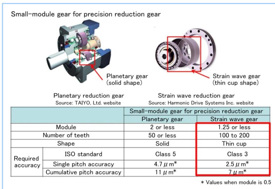
Figure 1 Features of planetary gears and strain wave gears
