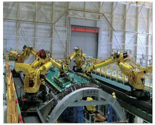
Figure 7 Handling robot
