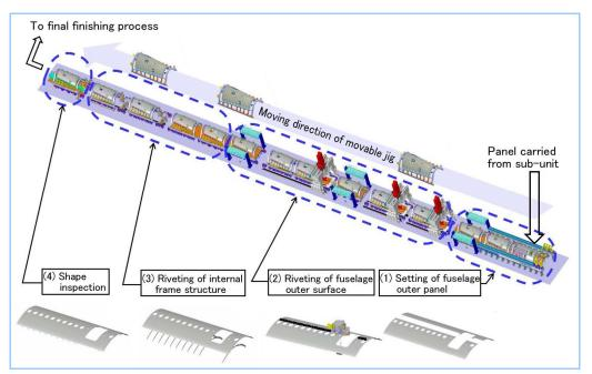
Figure 3 MPAL process schematic drawing
