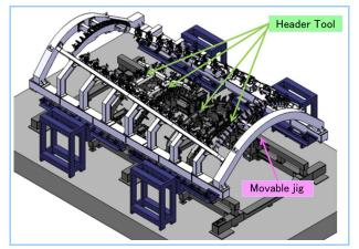
Figure 6 Header tool and movable jig
