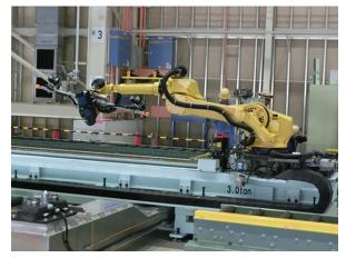
Figure 8 Shape inspection equipment
