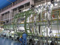
Figure 1 Fuselage division schematic drawing Figure 2 Conventional stationary jig
