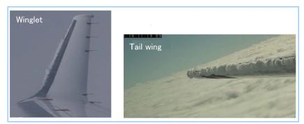
Figure 6 Icing state in natural icing test
