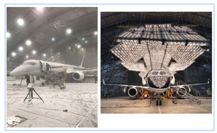
Figure 7 Extreme cold and heat test
