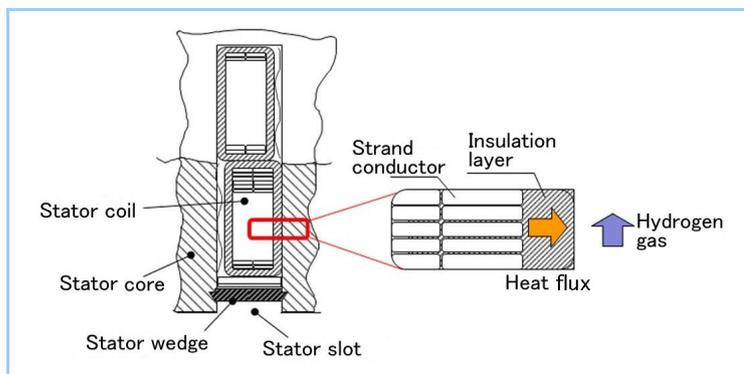
**Figure 3** Cross section of stator coil
