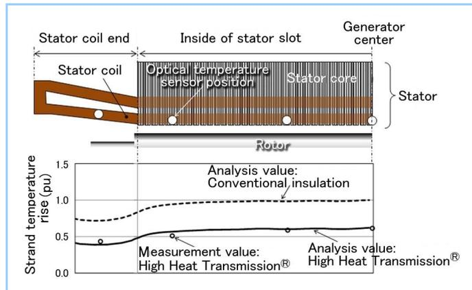
Figure 5 Analysis of stator coil strand temperature and measurement results
