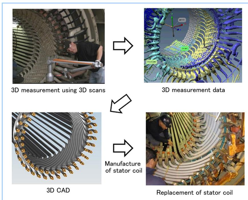
**Figure 9 Replacement of stator coil of generator manufactured by other companies**
