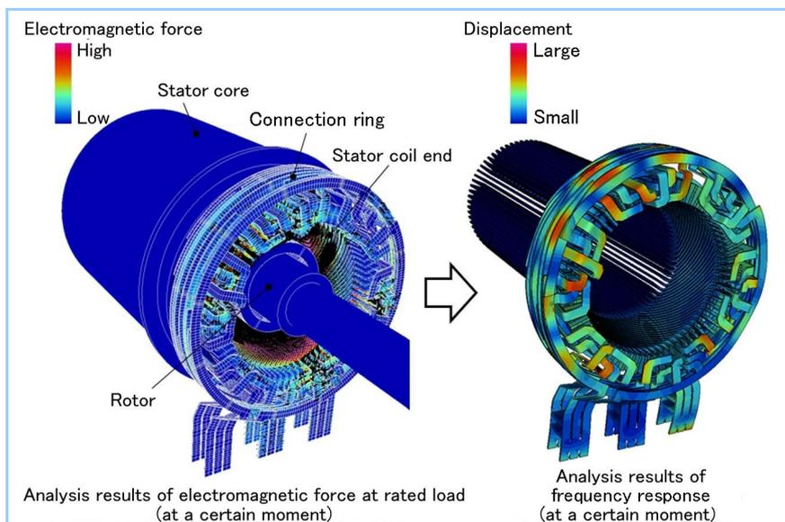
**Figure 2** Frequency response analysis with electromagnetic force analysis at stator coil end
