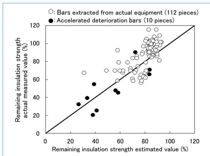
**Figure 7 Comparison between values estimated by remaining insulation life evaluation method and measured values**
