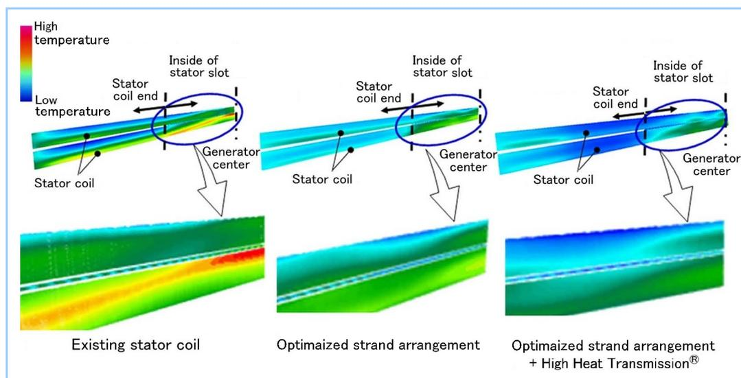
**Figure 6** Analysis results of stator coil temperature
