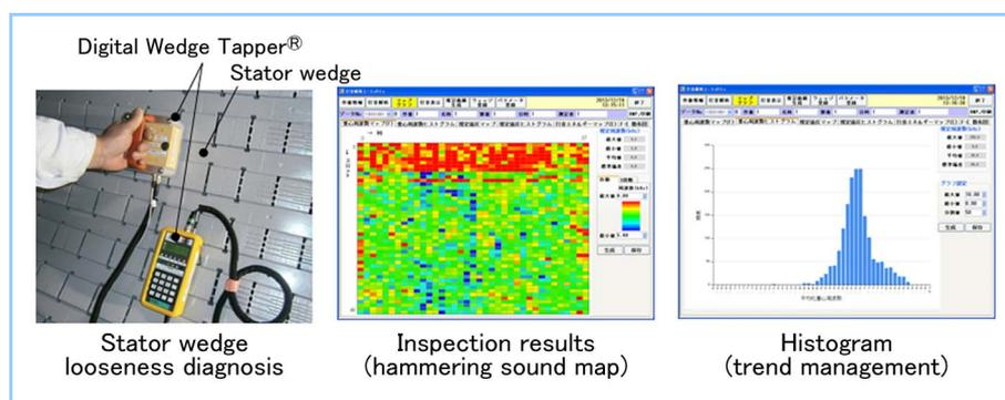
**Figure 8 Stator wedge looseness diagnosis (Digital Wedge Tapper<sup>®</sup>)**
