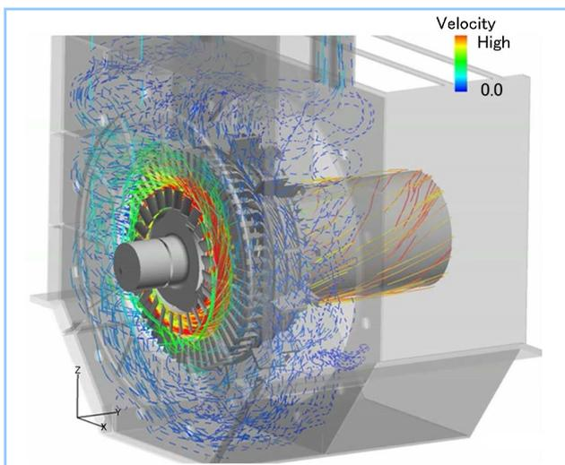
**Figure 1** Fluid analysis from ventilation fan to periphery of stator coil end (flow line distribution)
