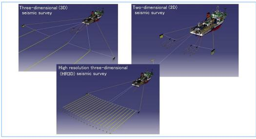
Figure 4 Three-mode multi-channel seismic survey system of the research vessel Kaimei
