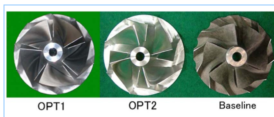
Figure 3 Comparison of baseline impeller and optimized impeller
