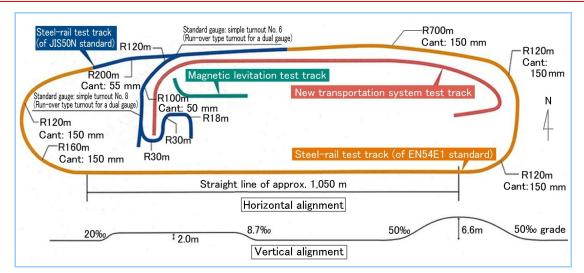
Figure 1 The track layout of MIHARA Test Center
