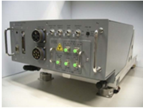
Figure 3 Outside Appearance of SHM Device
