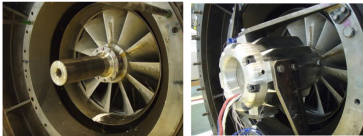
Figure 8 Drive shaft and coil installed on MET83MA turbocharger
