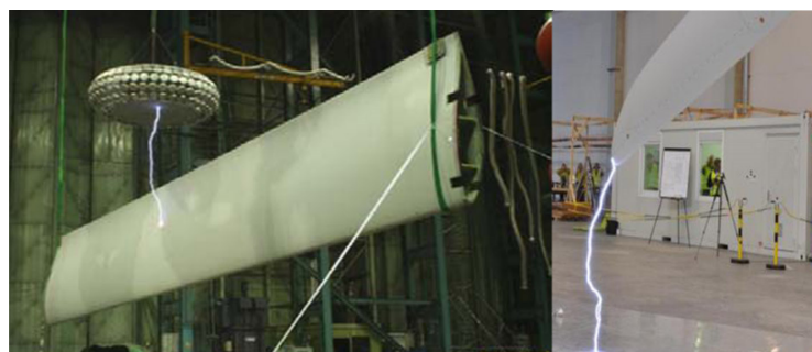
Figure 8 Appearance of the lightning test for the blades
