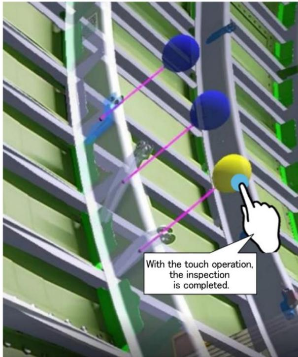
Figure 3 Record of inspection results (touch operation)
