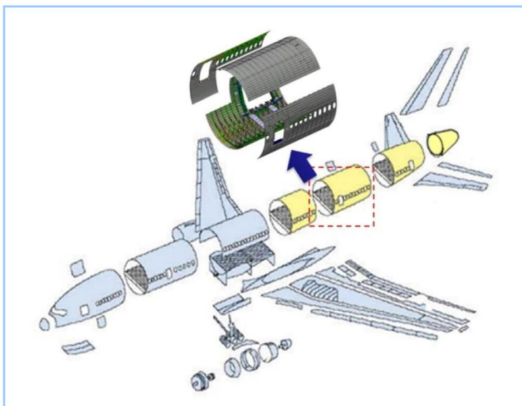
Figure 1 Aircraft fuselage panels
