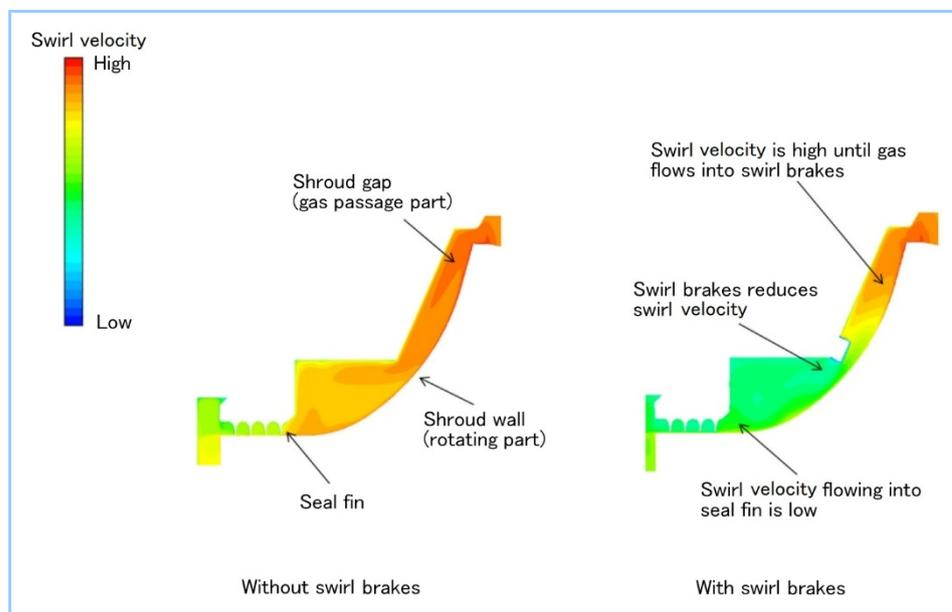
**Figure 8 Swirl velocity distribution in shroud gap**
