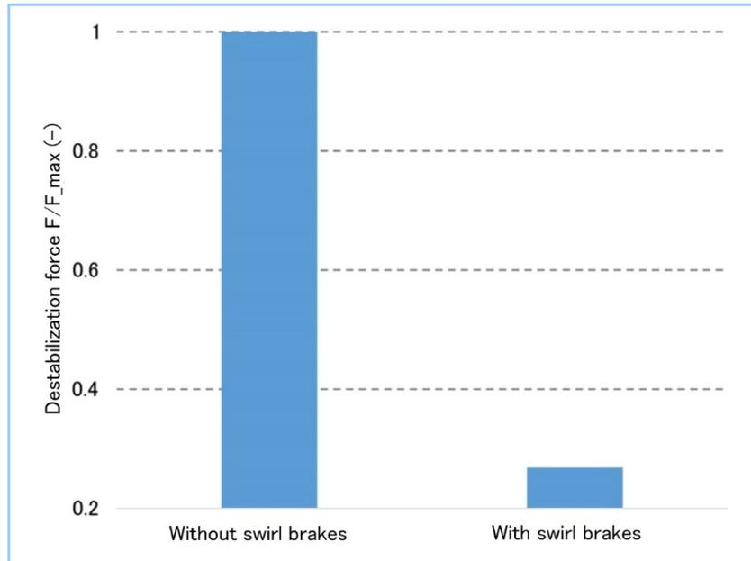
**Figure 7 Comparison of destabilization force with and without swirl brakes**
