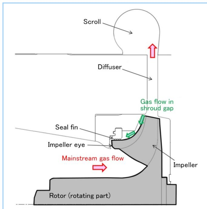
Figure 1 Centrifugal compressor
