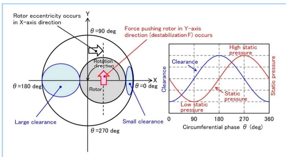
**Figure 4 Schematic of circumferential clearance distribution and static pressure distribution caused by rotor eccentricity**
