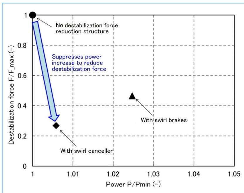
**Figure 10 Relationship between power and destabilization force with and without destabilization force reduction structure**
