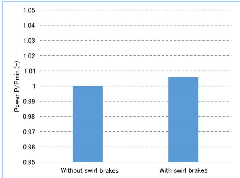
**Figure 9 Comparison of power with and without swirl brakes**
