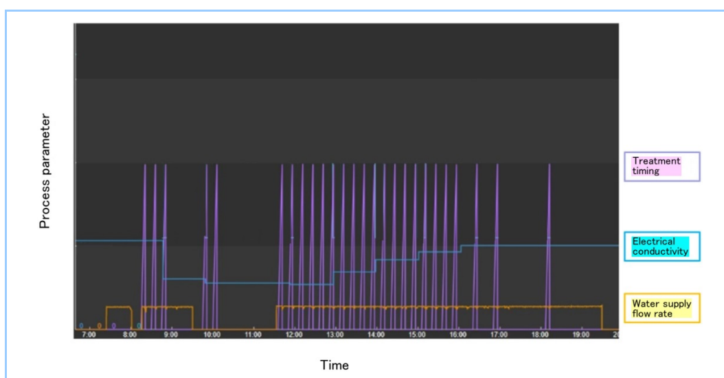
Figure 5 Water washing bath monitoring screen (correlation analysis)
