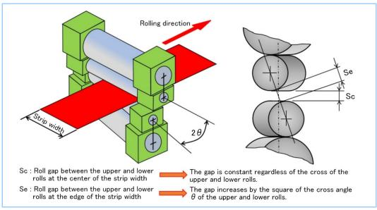
Figure 2 Principles of PC Mill
