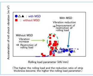
Figure 4 High load rolling by MSD
