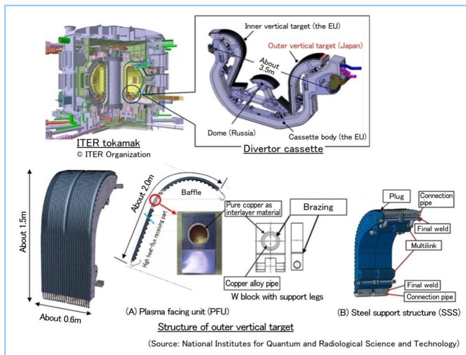
**Figure 6** Concept of ITER divertor and OVT (Over Vertical Target) structure
