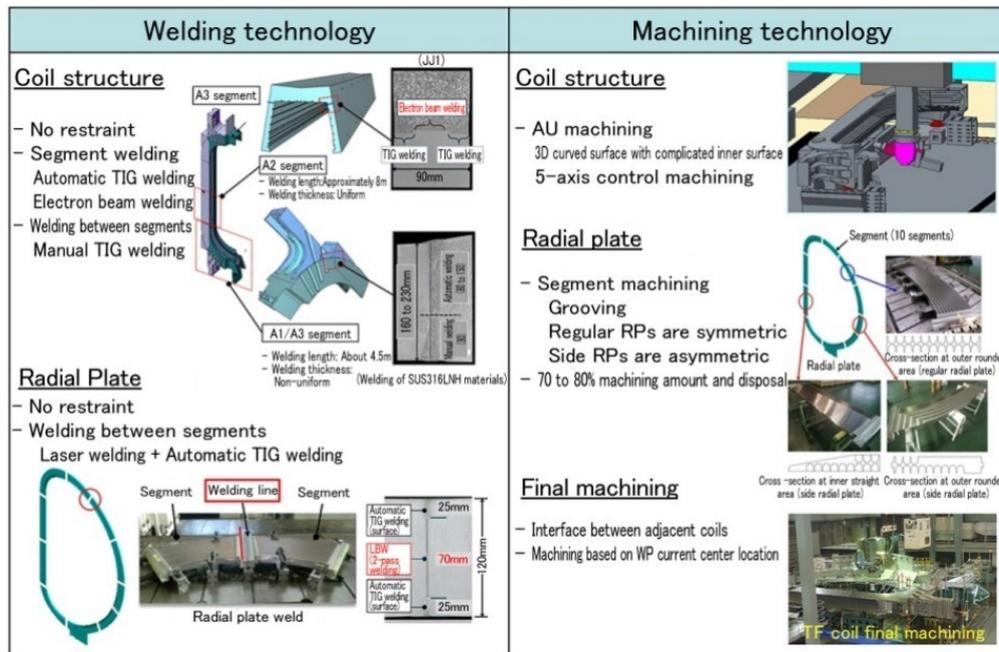
**Figure 2** Typical manufacturing technology used for TF coils
