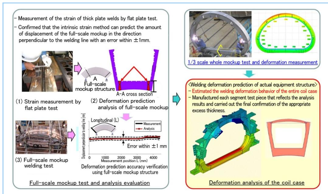
**Figure 4 Establishment of integration welding technology (full-scale mockup test and sensitivity analysis)**
