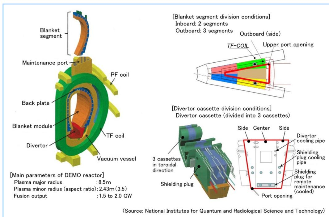
**Figure 12** Concept of reactor structure of DEMO reactor
