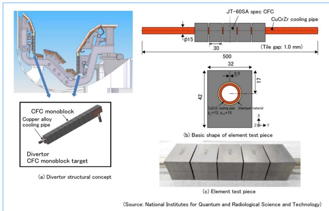
Figure 14 Structural concept and shape of element test piece of JT-60SA divertor
