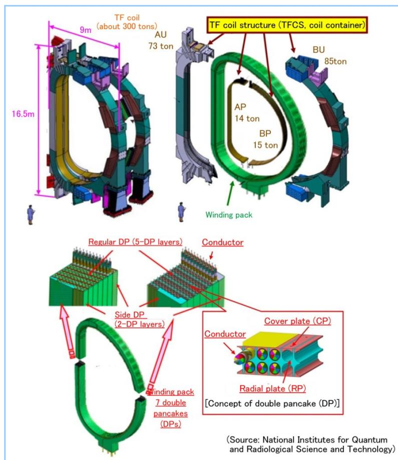
**Figure 1** Concept of toroidal field coil
