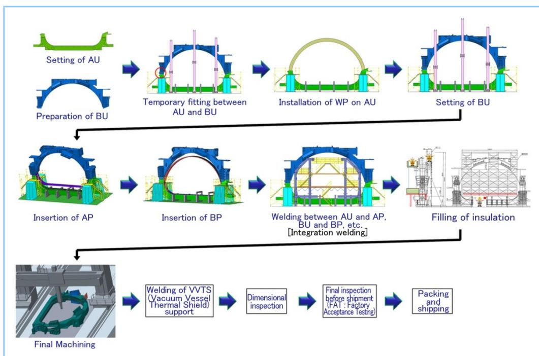
**Figure 3** Schematic flow of integration process
