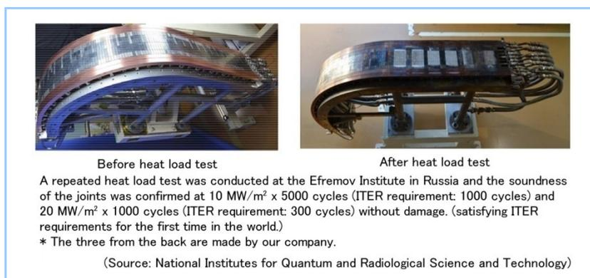
**Figure 7 High heat flux test of full W-PFU prototype of outer divertor**
