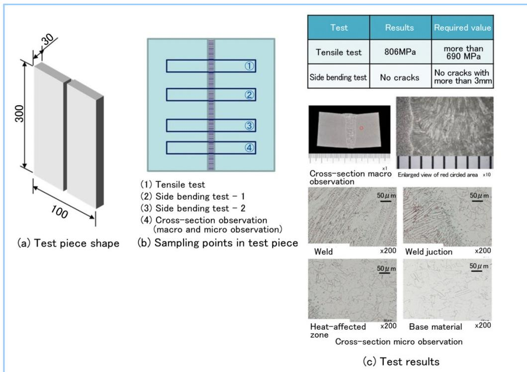
**Figure 10** Weldability test of XM-19
