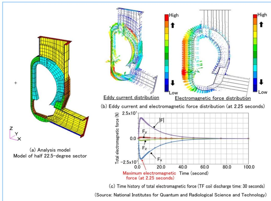
**Figure 13** Electromagnetic force analysis on vacuum vessel
