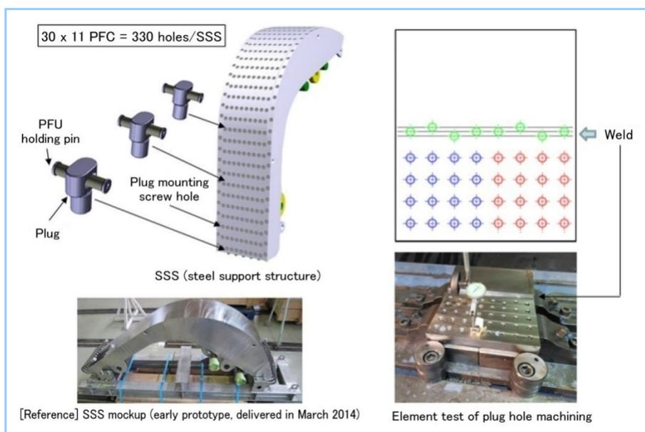
**Figure 11** Element test of machining screw holes on SSS
