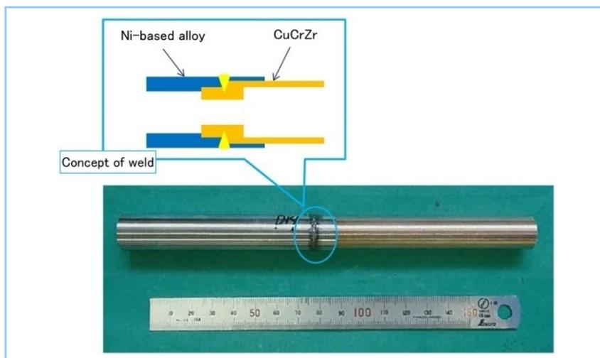
Figure 9 Element test of dissimilar welding (CuCrZr and Ni-based alloy)
