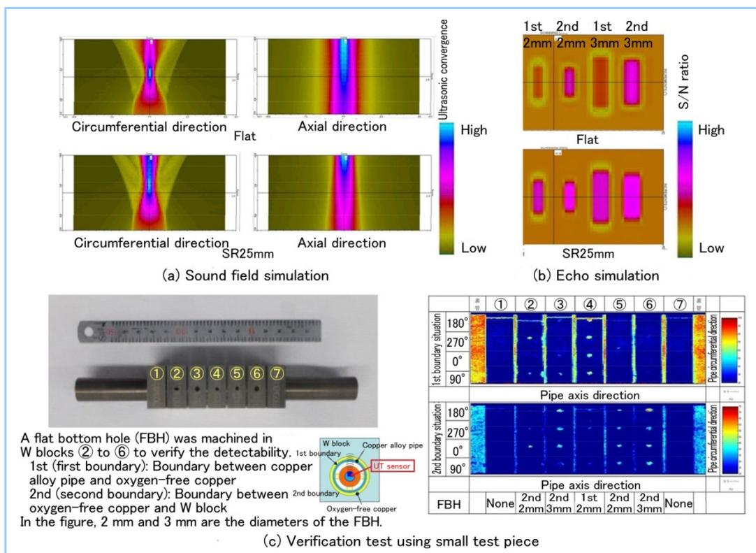
Figure 8 Preliminary tests of performance and sensitivity of UT for brazing joint
