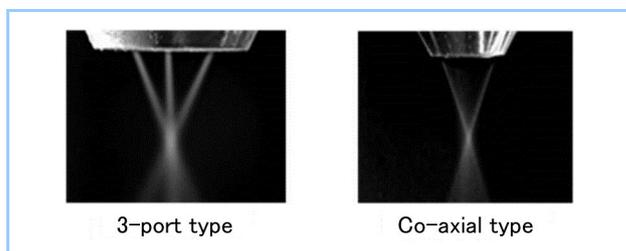
**Figure 6** State of powder convergence by each nozzle
