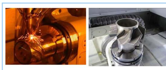
**Figure 9** Scene of the additive manufacturing of the blade profile (left) and the finished product (right)
