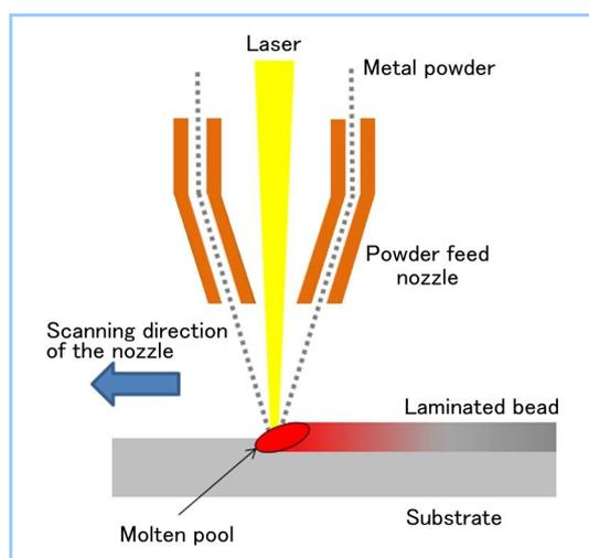
**Figure 1** Deposition-type additive manufacturing method
