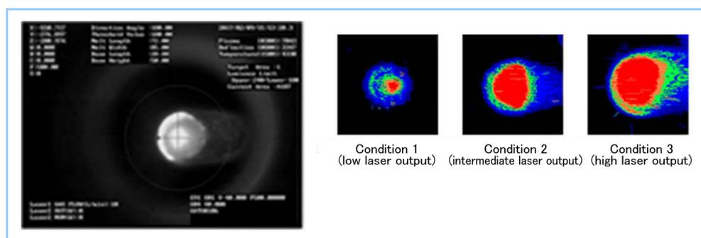
**Figure 5** Images of the molten pool (change of the molten pool size and temperature distribution by laser output level)
