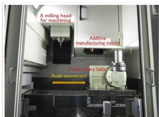
**Figure 2** Inside of the additive manufacturing system
