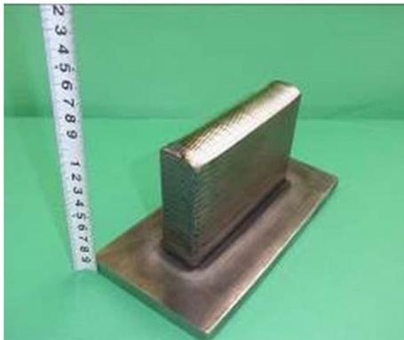
**Figure 11** Titanium alloy specimen for additive manufacturing
