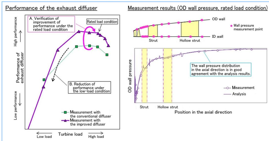
Figure 8 Verification of performance of the improved turbine exhaust diffuser
