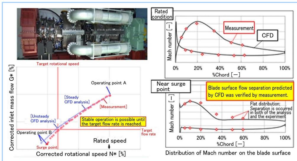
Figure 3 Verification of 8-stage compressor surge test and simulation
