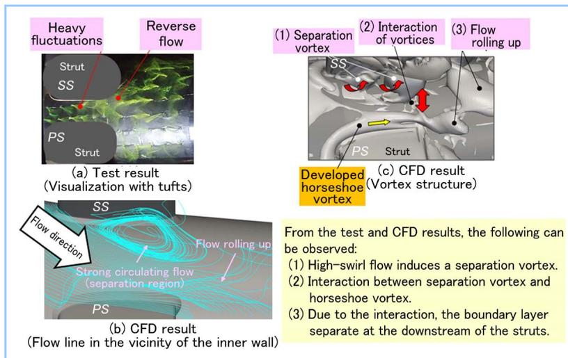
Figure 9 Flow structure in the diffuser strut inner wall (low-load condition)
