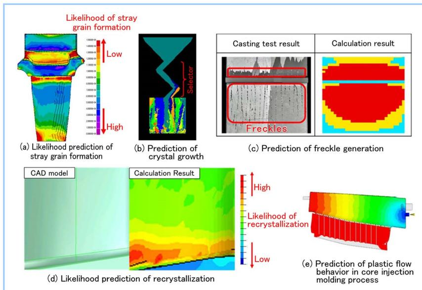
Figure 22 Simulation (calculation) results for each casting process
