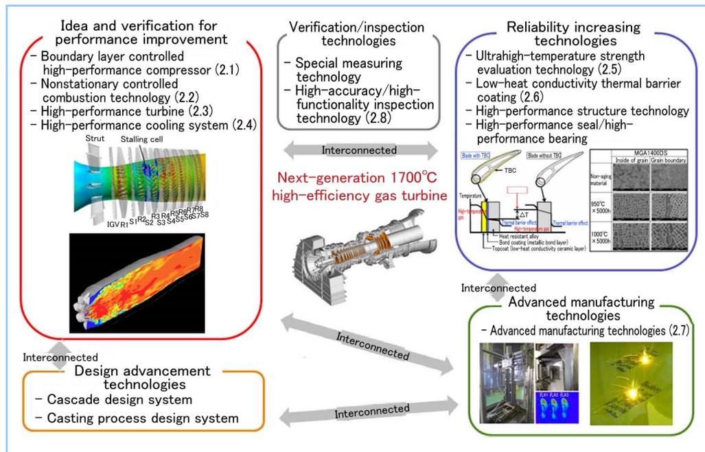
**Figure 2** Development of key technologies for ultrahigh-temperature gas turbines
