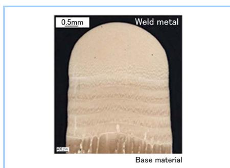
Figure 19 Cross section of the weld bead microstructure
