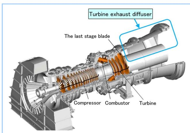
**Figure 7 Turbine exhaust diffuser**
