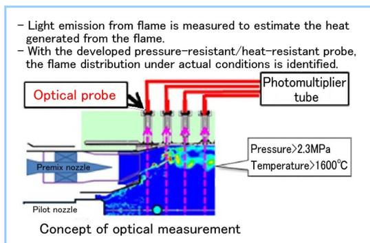
**Figure 5 Overview of the optical measurement for the inside of a combustor**
