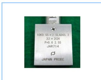
**Figure 24** Appearance of the matrix array UT probe
