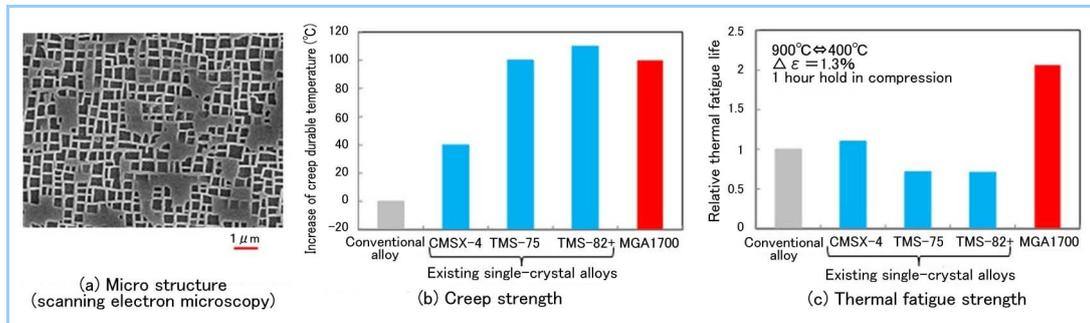
Figure 21 Micro structure and high-temperature mechanical properties of the developed alloy
