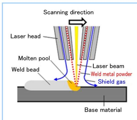
Figure 17 Schematic diagram of LMD
