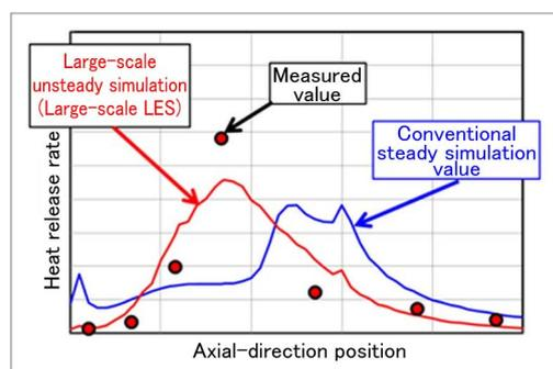
**Figure 6 Measurement of the combustor heat release rate in the high-temperature and high-pressure field**
