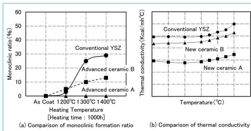
Figure 15 Measurement results of high-temperature stability and thermal conductivity of the topcoat materials (sintered bodies)
