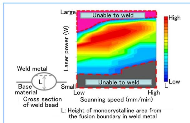
Figure 18 Relationship between the LMD condition and range of monocrystalline growth
