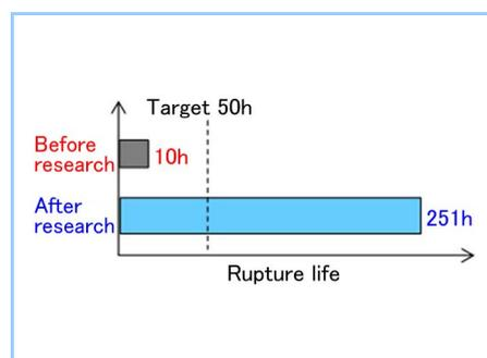
Figure 20 High-temperature creep rupture test results
