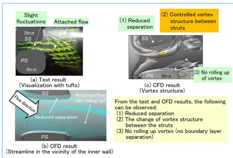
Figure 10 Effects in cases where the vortex structure is controlled (low-load condition)
