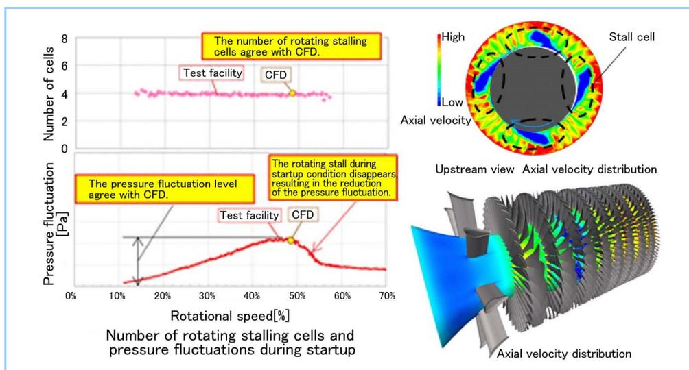
Figure 4 Comparison of measurement and simulation for rotating stall phenomena at startup condition of 8-stage compressor
