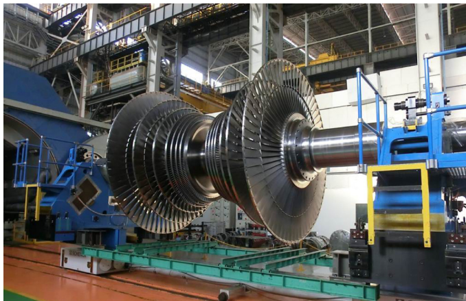
Figure 2 Turbine high-speed balancing facility
