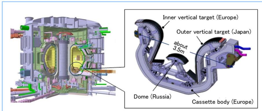
**Figure 11 Structural concept of an ITER divertor**
