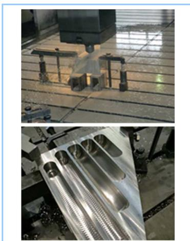
**Figure 5 Primary tests for RP grooving**
