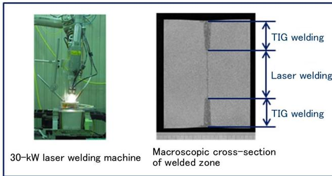
**Figure 4 Primary tests for RP welding**
