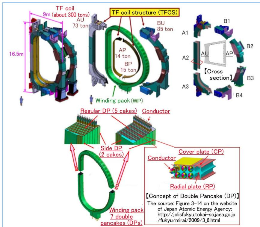
**Figure 1** Concept of toroidal field coil structure
