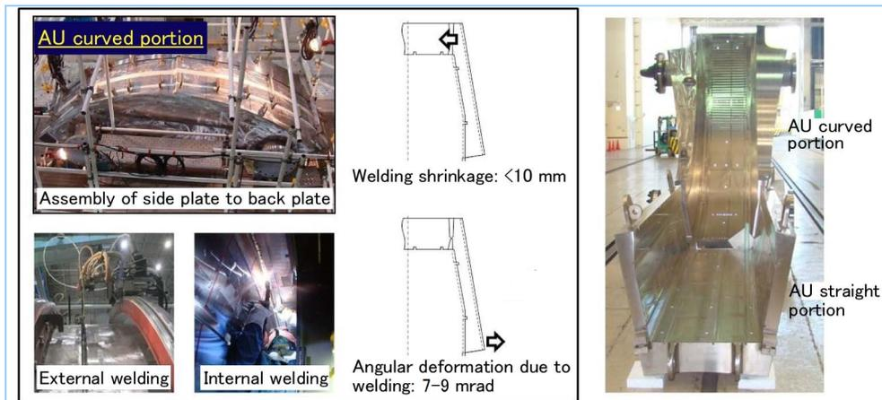
Figure 3 Full-scale, partial mock-up test (AU curved and straight portion)
