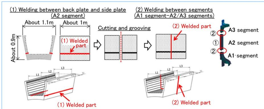
Figure 2 Small-scale mock-up test
