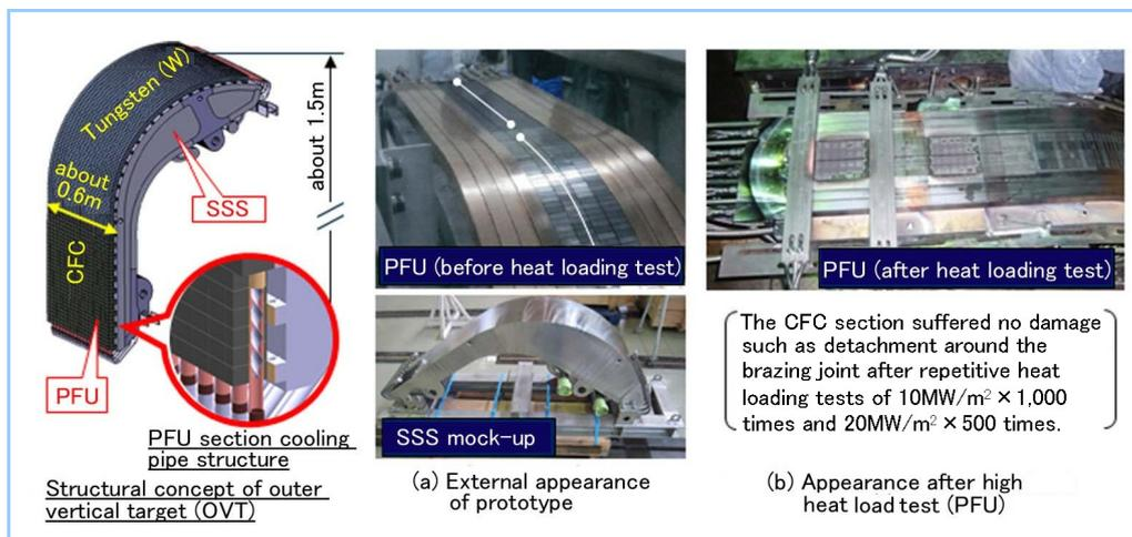
**Figure 12 Trial manufacture and tests of an outer vertical target prototype of a divertor**
