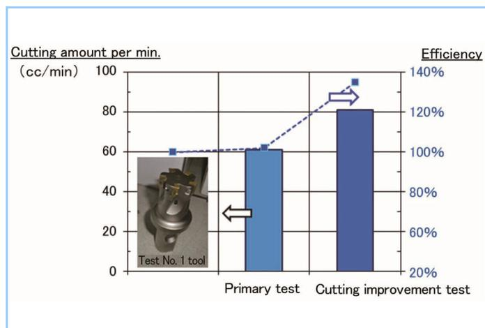
**Figure 6 Improvement of cutting performance in Test No. 1 tool (Table 3)**
