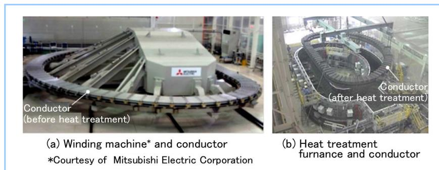
**Figure 9** Example of special equipment for manufacturing TF coils
