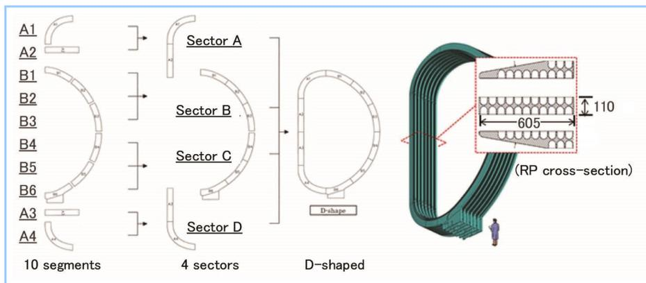
**Figure 7** Concept of RP structure (Courtesy of: The Japan Atomic Energy Agency)
