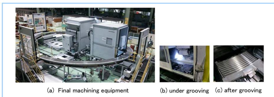
**Figure 8** Final machining of sRP full-scale mock-up
