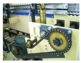
Figure 2 Drive components of conventional packaging machine Mechanically linked system is employed.
