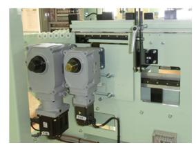
Figure 3 Drive components of new packaging machine Multi-servo driving system is employed.
