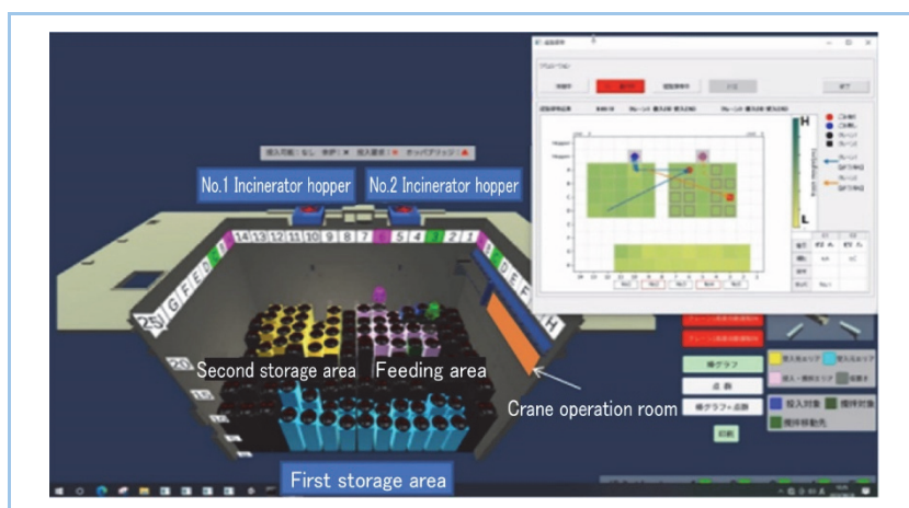
Figure 2 Advanced automated crane operation system
