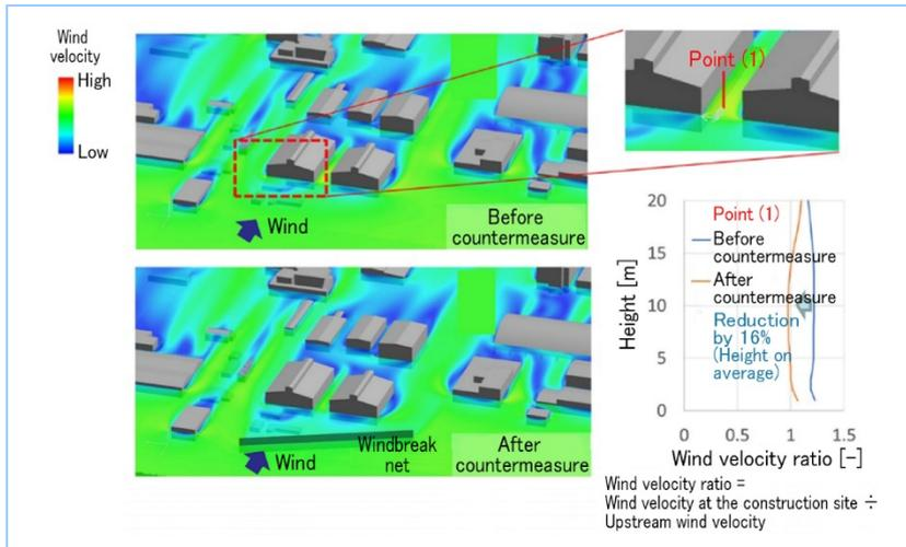
**Figure 7 Strong wind damage simulation**
