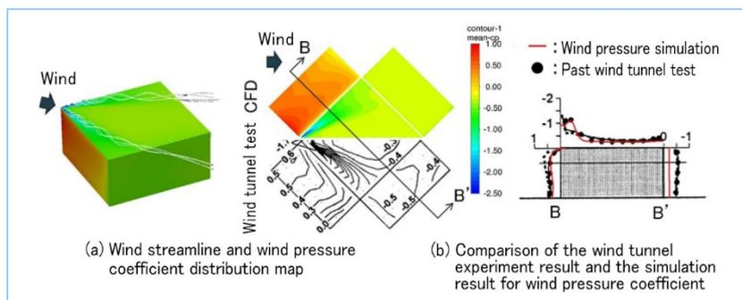
**Figure 3** Validation result of wind pressure simulation<sup>(5)</sup>
