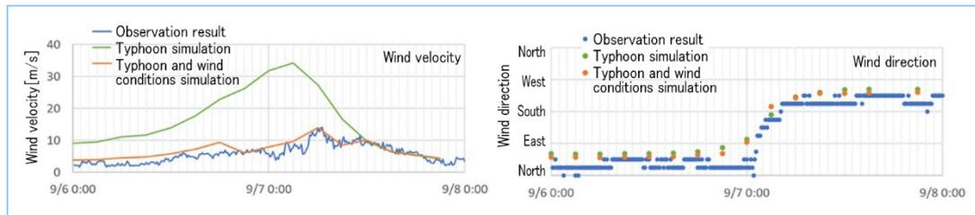
**Figure 2** Validation result of typhoon simulation and wind conditions simulation
