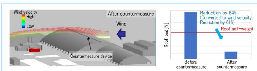
Figure 6 Roof uplift damage simulation (after countermeasures)
