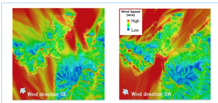
**Figure 8 Design wind velocity map**
