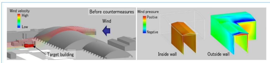
Figure 5 Roof uplift damage simulation (before countermeasures)
