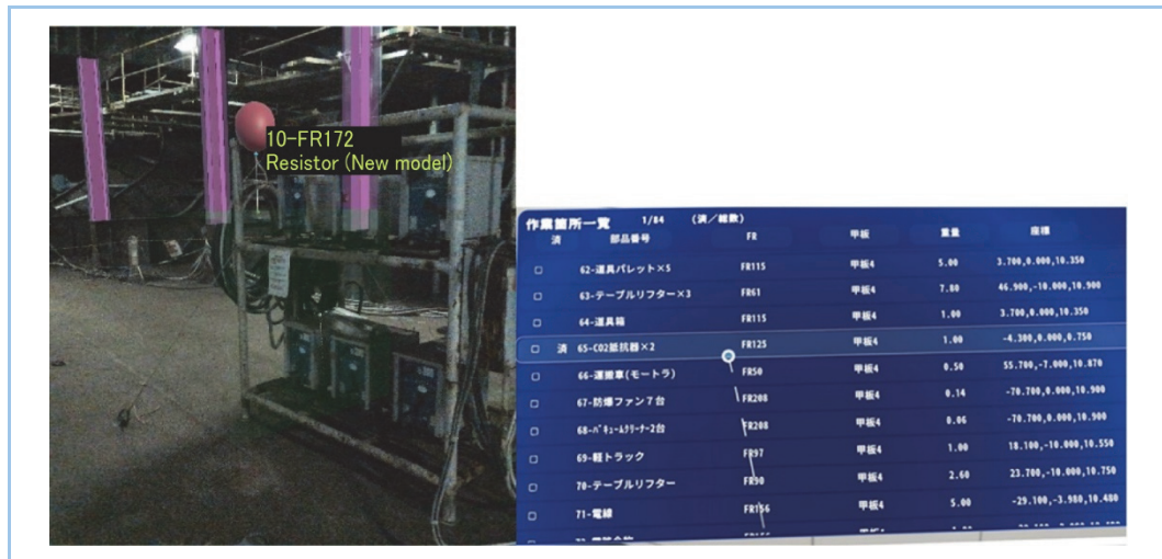
Figure 5 Superimposed display of cube and balloon object over loaded objects
