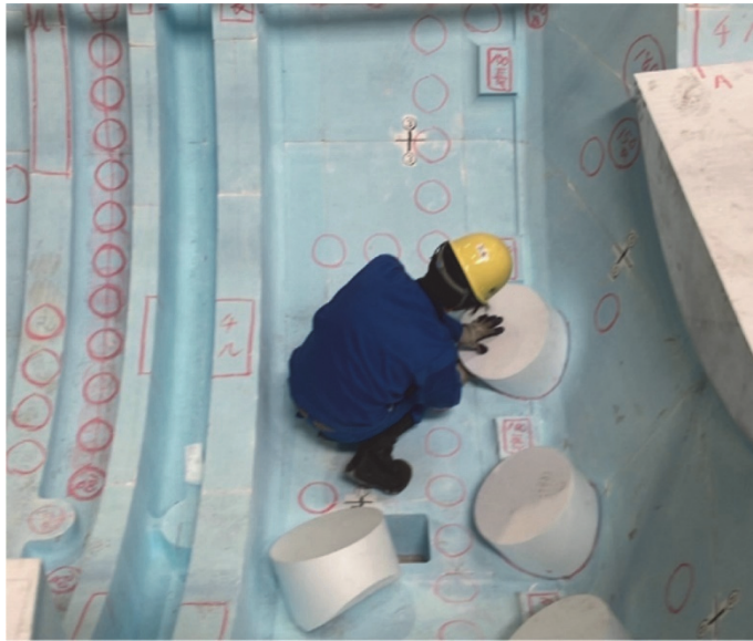
Figure 2 Marking work on a mold pattern
