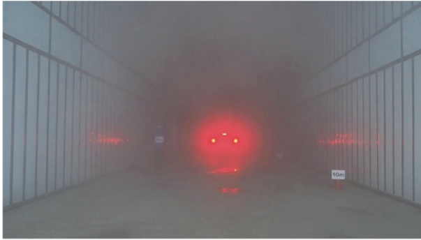
Figure 7 Fog emulation in demonstration test facility Testing situation in which fog is generated within demonstration test facility
