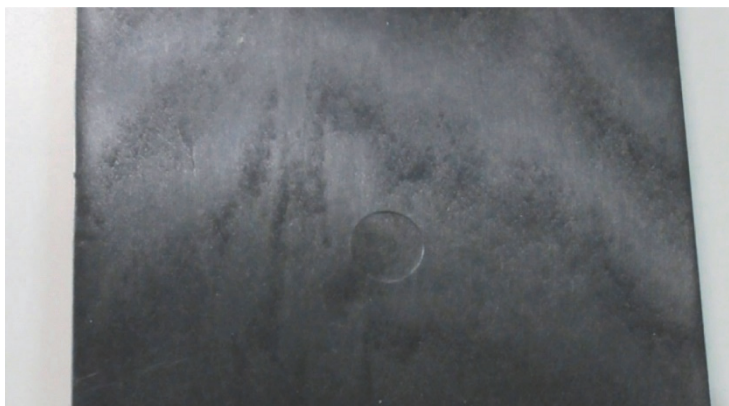
Figure 7 Appearance quality of injection-molded part using recycled carbon fibers
