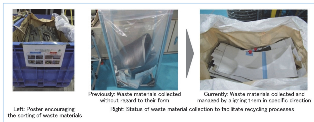
Figure 2 Management of waste composite materials
