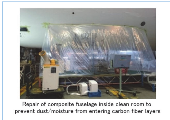
Figure 1 Repair of damage to fuselage made of composite materials*
