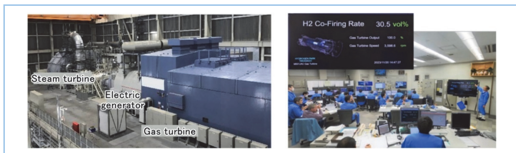
Figure 5 MHI's GTCC demonstration power generation plant's latest JAC gas turbine and central control room
