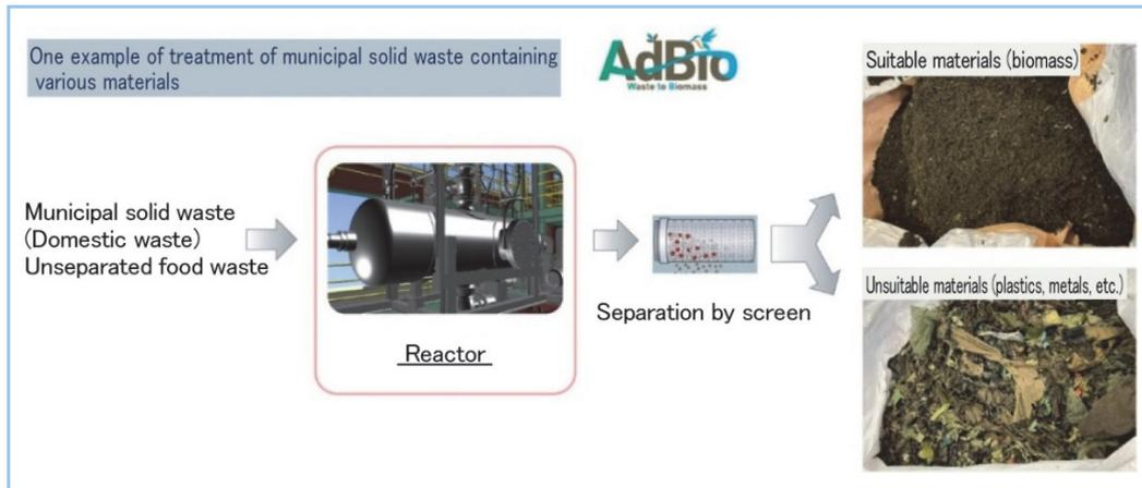
**Figure 5 High efficiency biomass collecting and recycling system**
