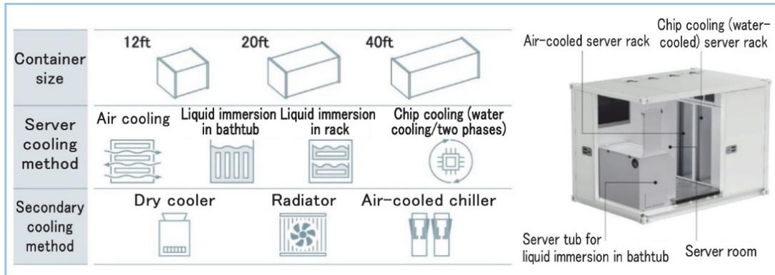
Figure 4 Container-type data center system<sup>(8)</sup>
