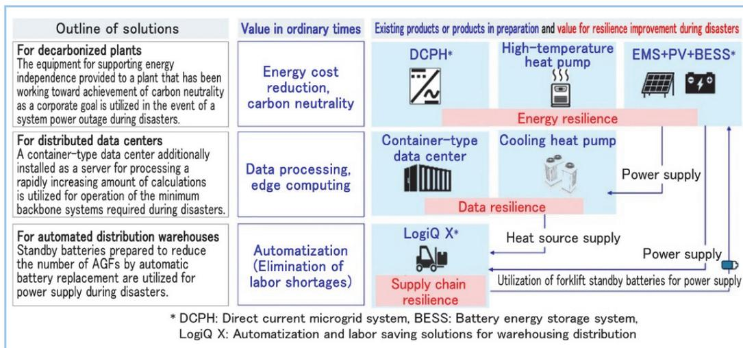
**Figure 3 Example of system that provides value both in ordinary times and during disasters by utilizing MHI Group products**
