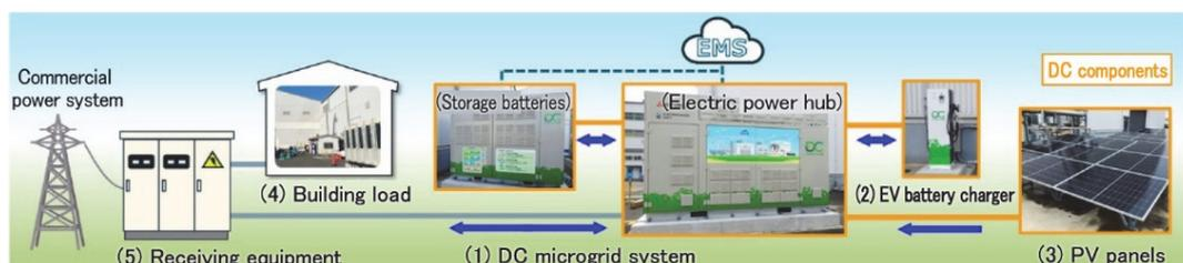
**Figure 6 DC microgrid system**
