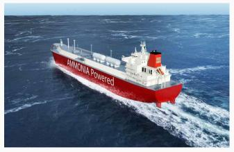
We completed the conceptual design of a Very Large Gas Carrier (VLGC) that can be converted from using LPG fuel to using ammonia fuel that does not emit  $CO_2$ .
