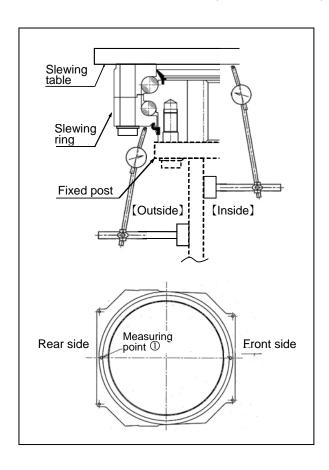
Fix the dial gauge on the outside surface of the fixed post as shown in the right figure, and apply the probe to the bottom surface of the outer ring of the slewing ring.
