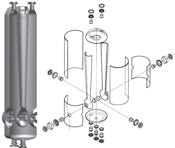
Figure 1: An exploded view of Superconducting QWR cavity.
