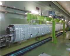
(a) Cold mass of STF2 cryomodule
