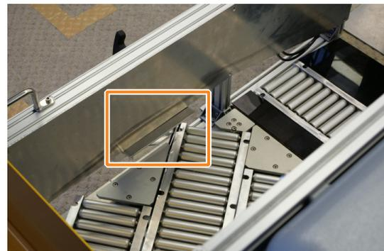
The cylinder is adjusted to expand and retract in 3 seconds. In other words, it should take about 3 seconds from the retracted state to the most extended state and from the extended state to the stowed position. Check whether the cylinder movement takes much more or less than 3 seconds. Depending on the position of the sub tracks when ASCENT is docked, the extended cylinder may collide and fail to connect properly. The sub tracks must be at an angle between 100° and 105°.
