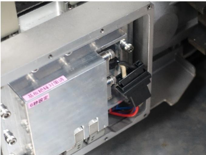
Next disconnect the smaller connector while pressing the tab on one side.
