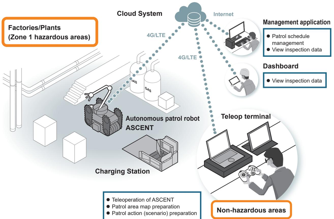
EX ROVR is designed to comply with Japanese guidelines for explosion protection and ATEX/IECEX, the explosion protection certification widely adopted in Europe and other parts of the world.
