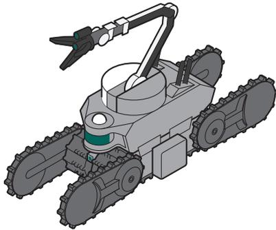
Robot that autonomously patrols inside a factory or plant to collect internal information. The system provides explosion-proof performance so that it cannot cause ignition in factories and plants where ignition is a hazard.
