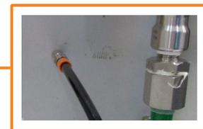
Connect the interlock check jig hose
