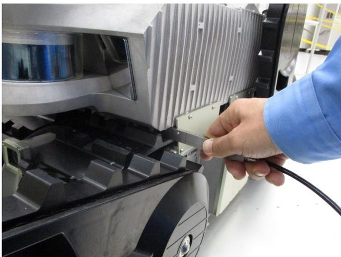
**9** Hook the concave tip of the interlock check jig onto the plug.
