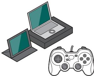
Terminal used to operate ASCENT. Does not have explosion-proof construction, and should be used in a non-hazardous area separate from the hazardous area where the ASCENT and Charging Station are installed. The terminal provides the following applications.
