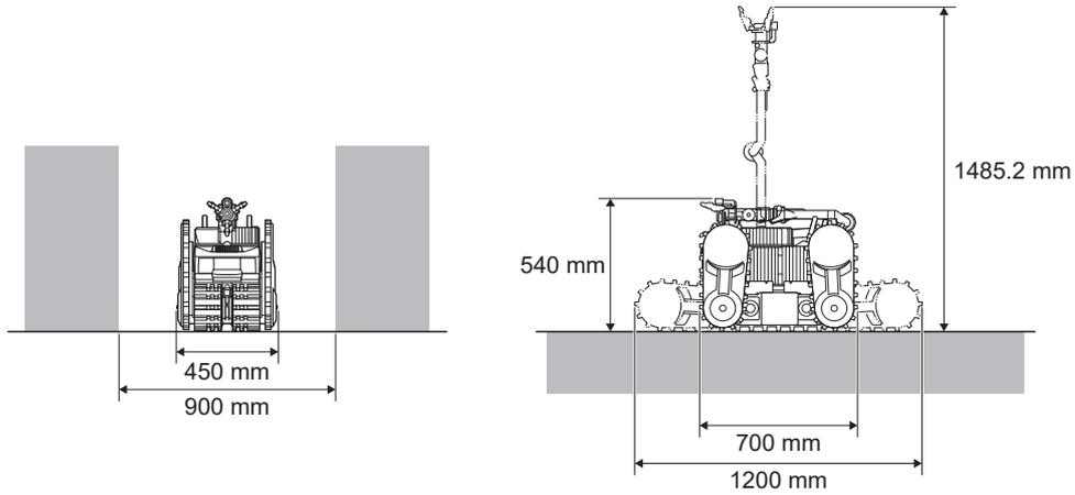
When turning in an aisle, available area must exceed the total length of ASCENT. Allow approximately 900 mm of space as shown in the figure on the right.
