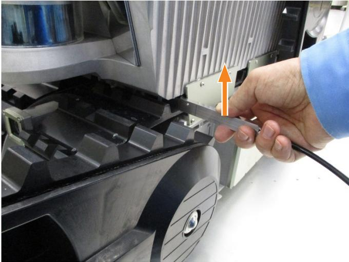
The “5PI1/Operation check jig pressure” should rise to about 8 kPa as ASCENT’s power shuts off.
