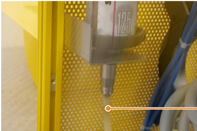
Pull the tube downward to remove it
