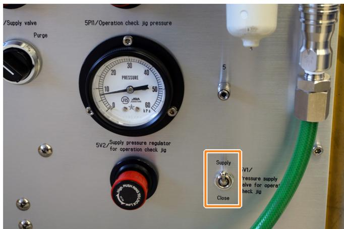
Air is discharged from the interlock check jig outlet, and the “5P11/Operation check jig pressure” reading drops.
