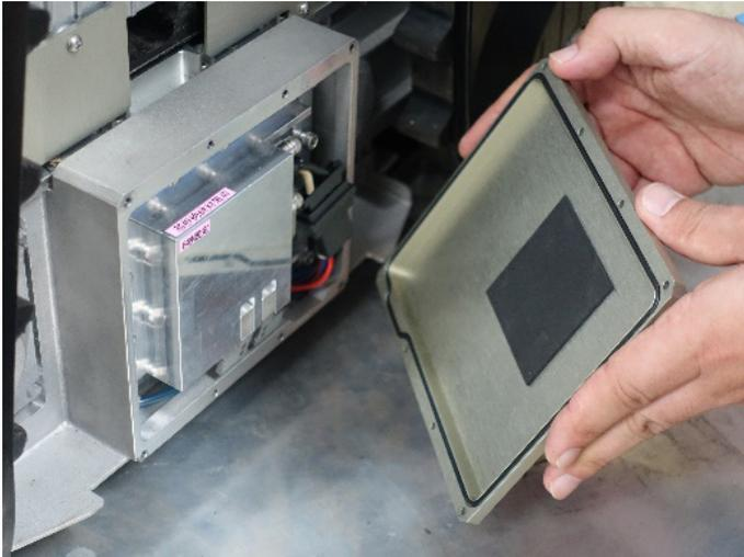
**4** Disconnect the two connectors between the battery and ASCENT's main unit.
