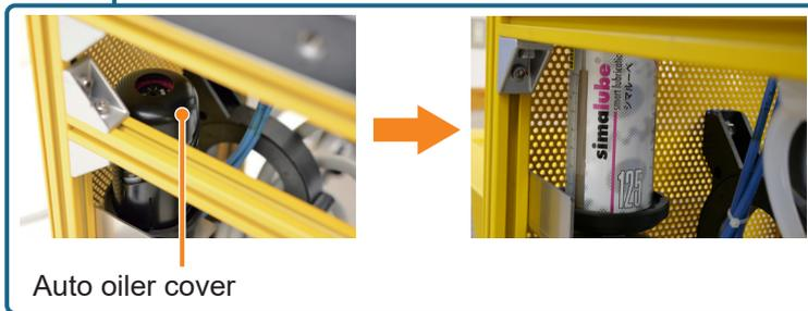
**6** Remove the tube connected to the bottom of the auto oiler.
