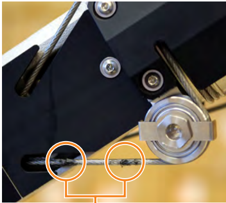
Minor cable damage
