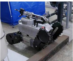
**8** After completely descending from the step, raise the front and rear sub tracks to return to the driving attitude.
