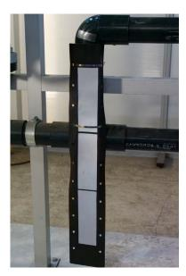
Marker size: 100 mm width x 600 mm length x 0.3 mm thick Three reflectors in the center of an aluminum plate (50 mm width x 160 mm length)
