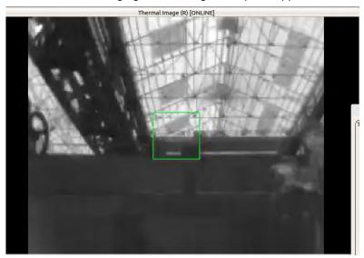
Depending on the attitude of the sub tracks, one may obstruct the view of the thermal imaging camera, and the heat source may not be visible or the image may be distorted. In that case, click the [Down (5°)] button to lower the sub tracks on the thermal imaging camera side.
