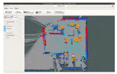
5 Return to the load-map motion properties screen and click the [Acquire Current] button. The position where ASCENT is currently located is set as the initial position attitude of the load-map motion.
