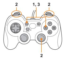
1 Press and hold the BACK button (Function) while pressing the X button (Synchronous/Independent).
