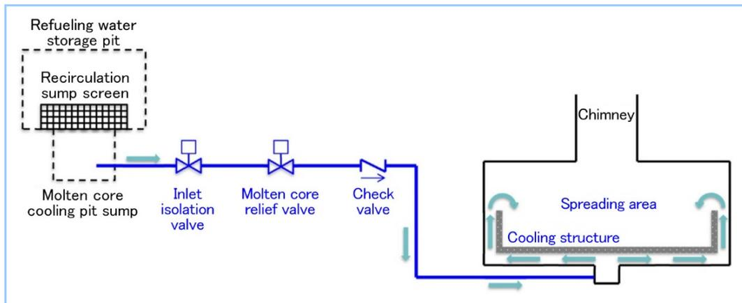
**Figure 3** Gravity injection into spreading area
