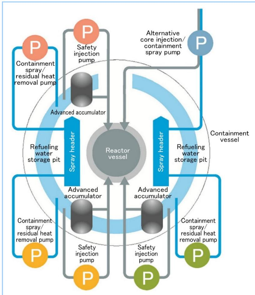
**Figure 1 Configuration of triple-redundant safety systems**
