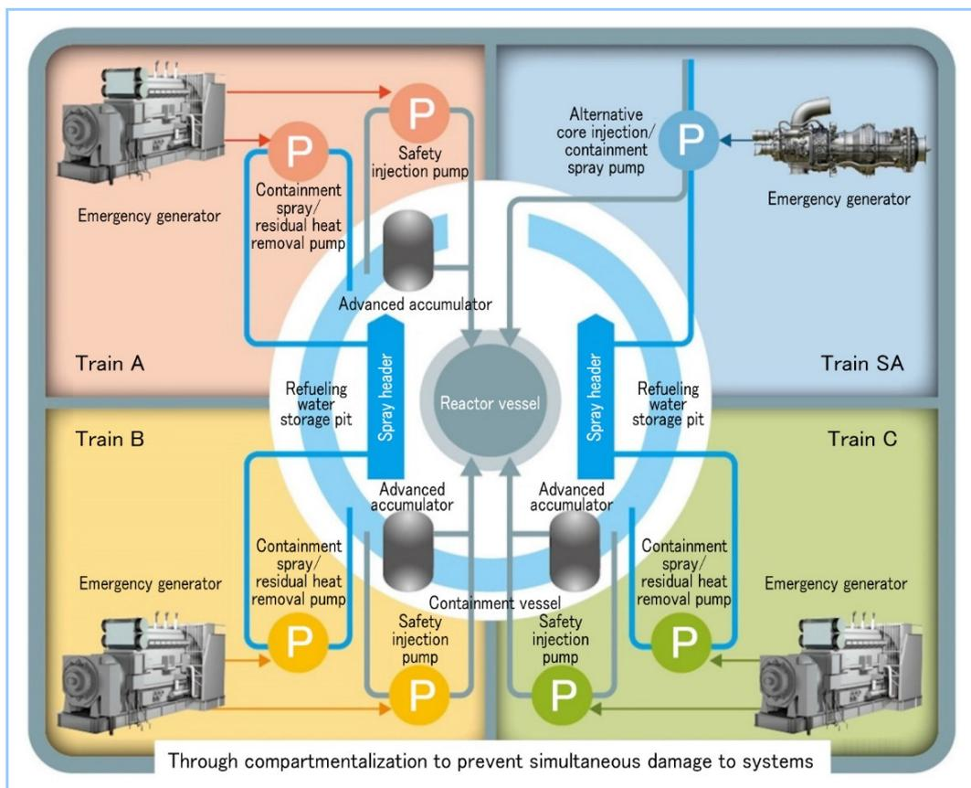
**Figure 4** Concept of compartmentalization
