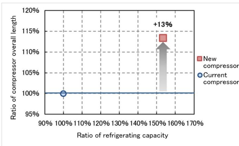
**Figure 2 Comparison of refrigerating capacity and overall length between current and new compressors**
