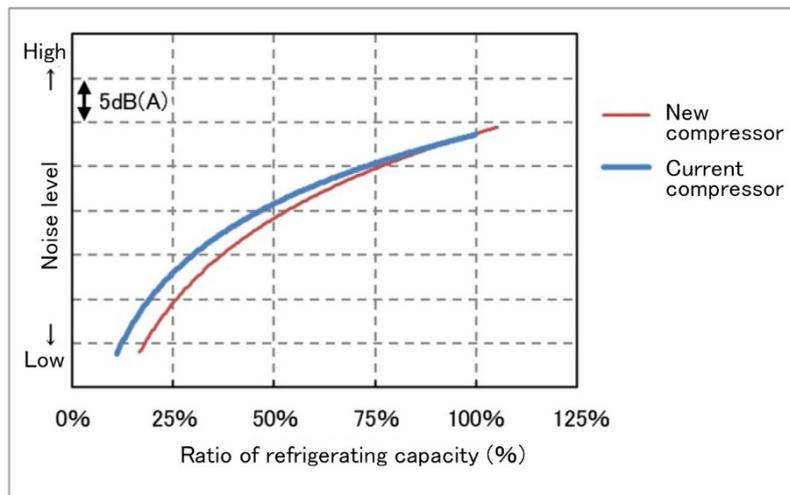
**Figure 3 Comparison of noise between current and new compressors**
