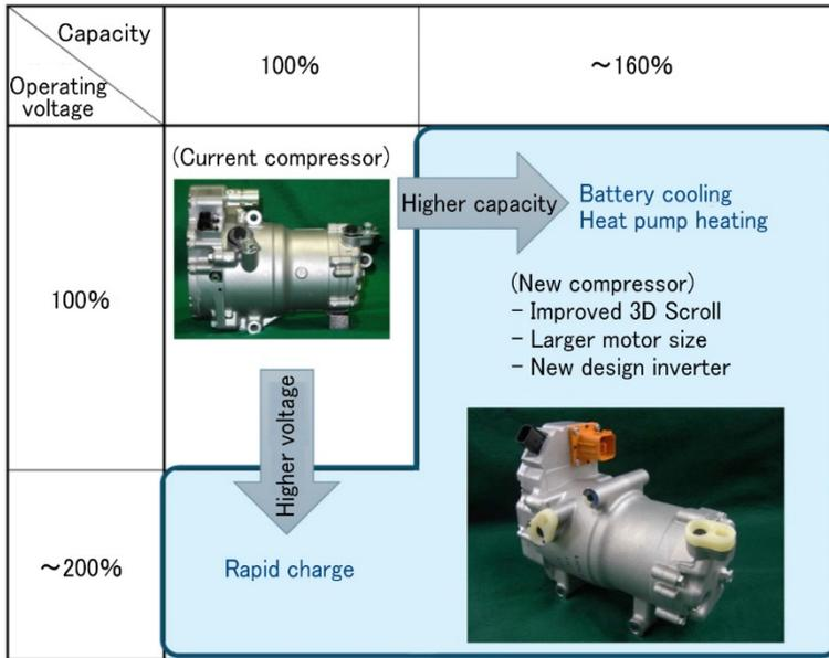
**Figure 1 Comparison of features and appearance between current and new compressors**
