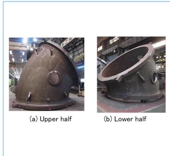
**Figure 6** Two-piece discharge elbow
