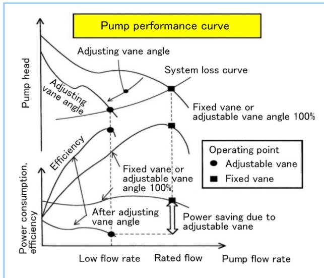
**Figure 3 Adjustable-vane circulating water pump performance curve**
