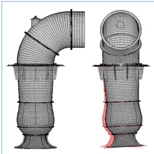
**Figure 5** Eigenvalue analysis results (structural system)
