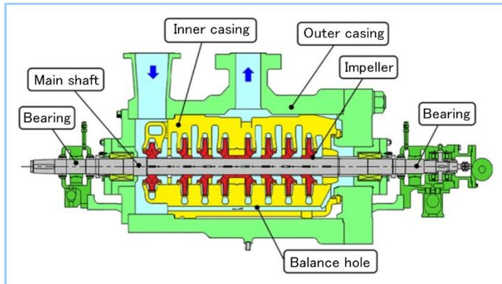
**Figure 8 High-pressure multi-stage pumps for the special safety facility of Japanese nuclear power plant**
