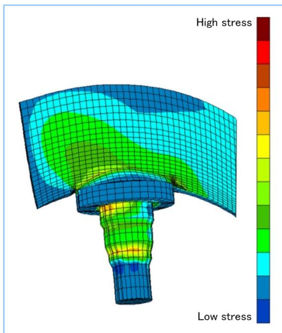
**Figure 4 FEM analysis results (stress generated on runner vane)**
