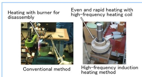
**Figure 10 Main shaft components disassembly tool using high-frequency induction heating method**
