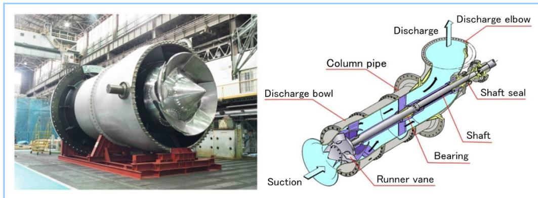
**Figure 1 Appearance and structure of large adjustable-vane circulating water pump**
