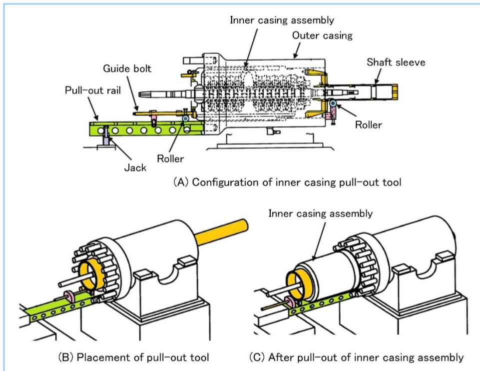
**Figure 9 Inner casing pull-out tool**
