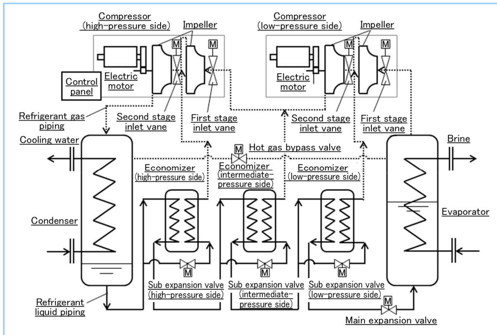
**Figure 2** Refrigeration cycle
