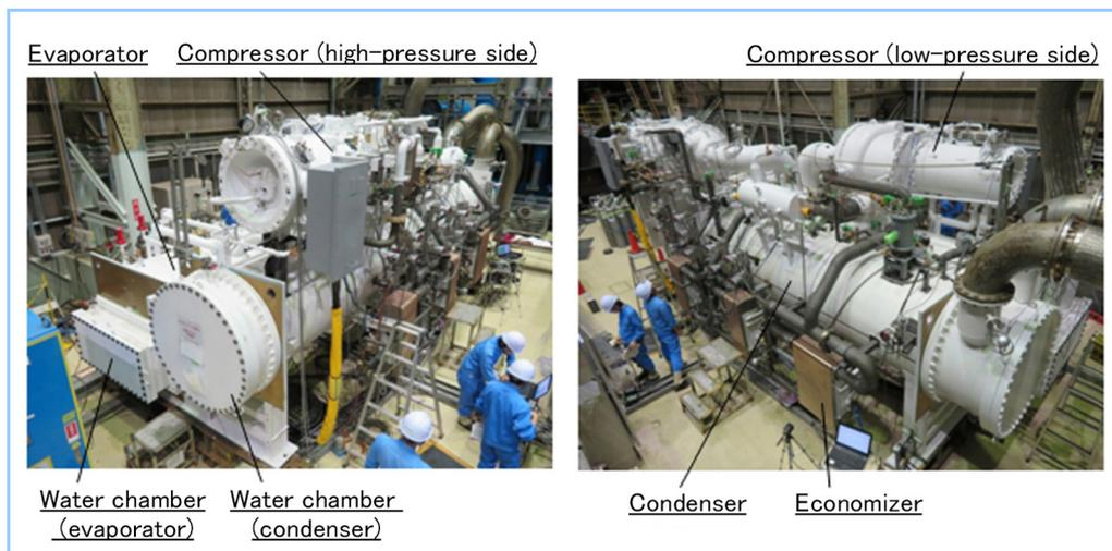
**Figure 3** External view (taken at time of factory trial operation)
