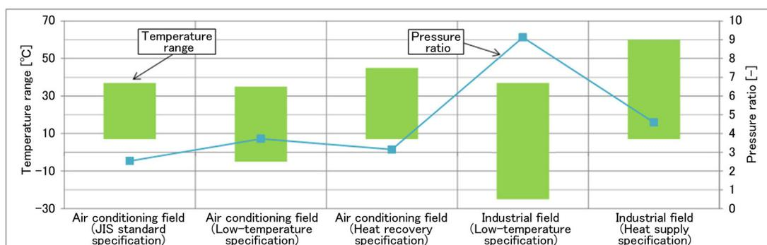
**Figure 1 Fluid temperature range and pressure ratio in air conditioning and industrial fields**
