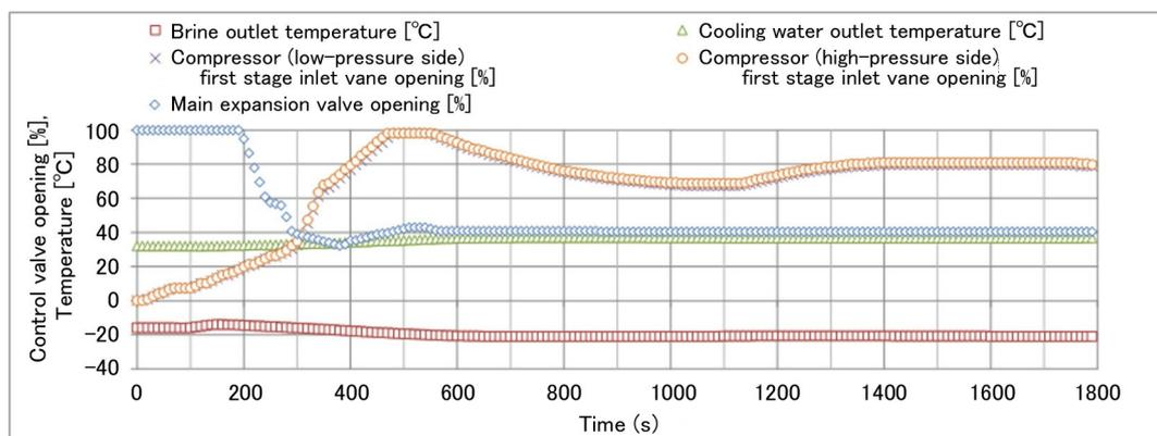
**Figure 4 Dynamic characteristic analysis result 1 (control valve opening, temperature)**
