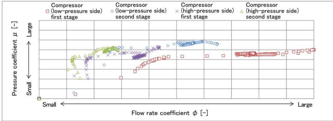
Figure 5 Dynamic characteristic analysis result 2 (flow rate coefficient, pressure coefficient)
