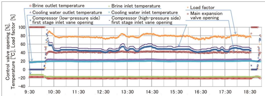
Figure 6 Operation data from startup to shut down
