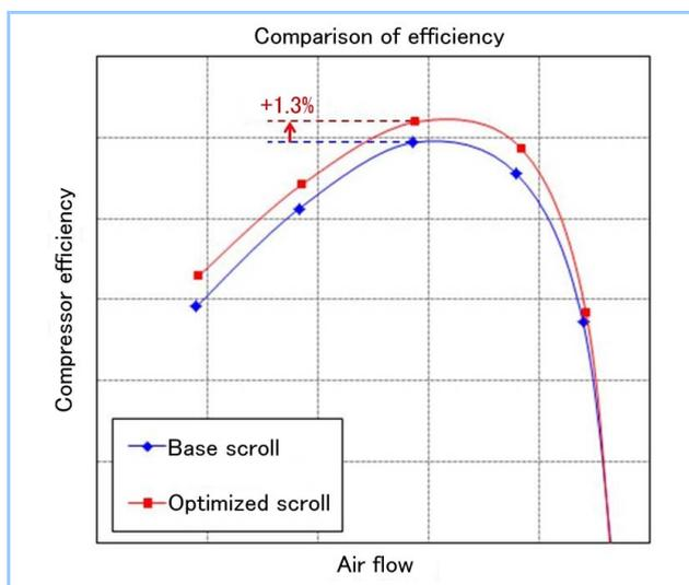
**Figure 13 Comparison of performance test results between before and after optimization of compressor scroll**
