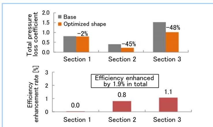
**Figure 15 Comparison of performance analysis results between before and after optimization of two-stage turbine**
