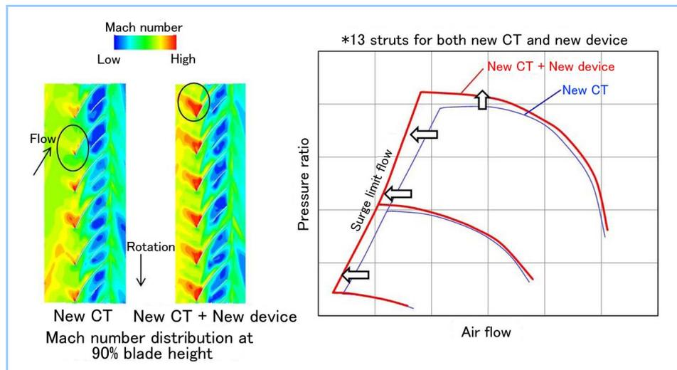
**Figure 9** Internal flow and performance of new device
