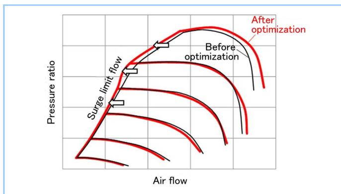
**Figure 11 Comparison of performance test results between before and after optimization of compressor impeller**
