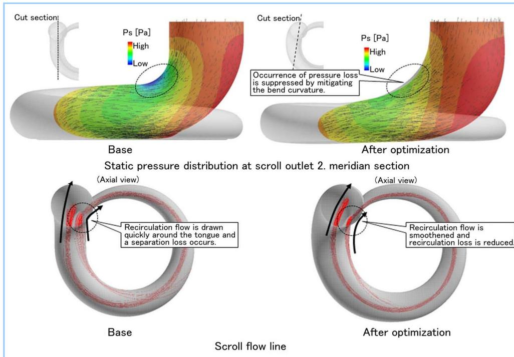
**Figure 12 Comparison of compressor scroll shape and internal flow between before and after optimization**
