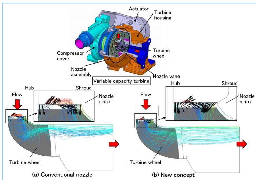
**Figure 1** Flow line and flow speed vector distribution at leading edge of rotor blade (small nozzle opening)
