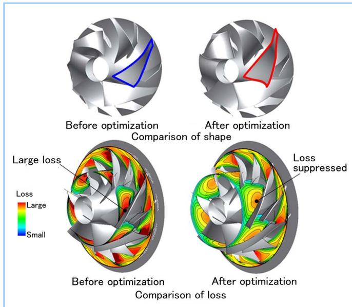
**Figure 10 Comparison of compressor impeller shape and internal flow between before and after optimization**
