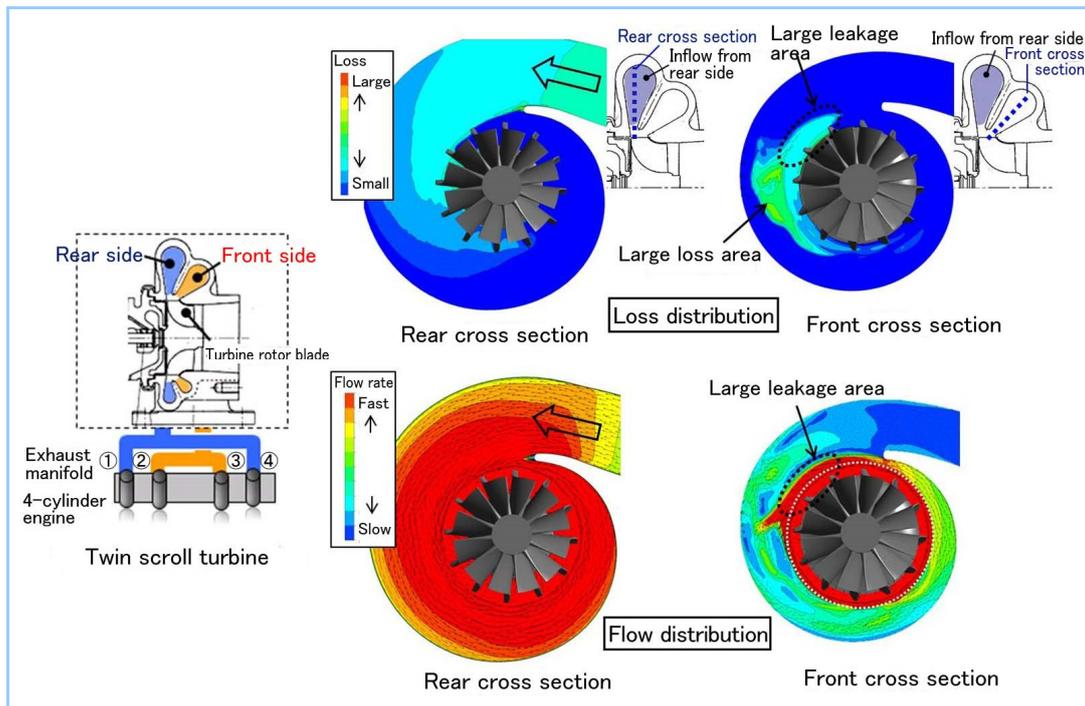
Figure 3 Turbine scroll internal flow in rear side inflow
