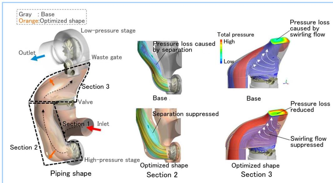
**Figure 14 Comparison of two-stage turbine shape and internal flow between before and after optimization**
