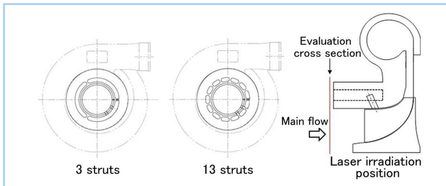
**Figure 6** Measurement of casing treatment internal flow
