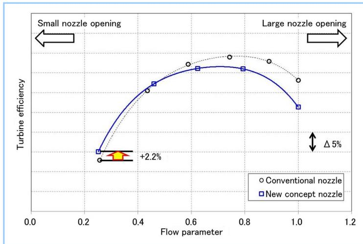
Figure 2 Results of VG turbine performance test
