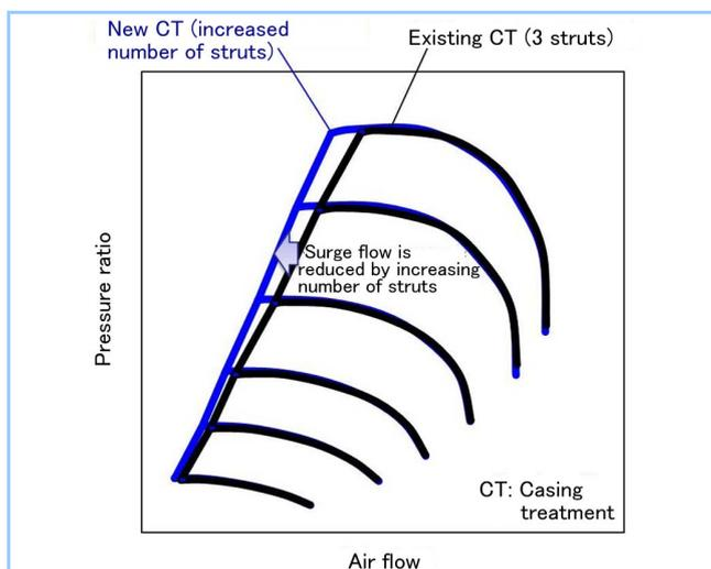
**Figure 5** Results of casing treatment performance test
