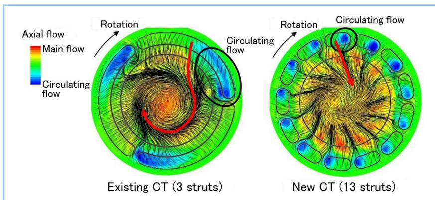
**Figure 7** Measurement results of casing treatment internal flow
