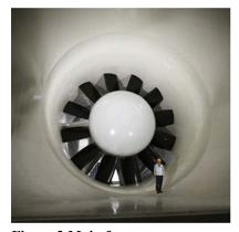
Figure 2 Main fan (upstream side)
