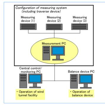
Figure 4 Wind tunnel operation and measurement system
